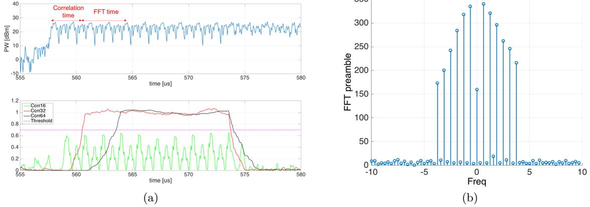
Figure 1: (a) Preamble time and correlations, (b) FFT shift of a preamble sent at 10MHz
