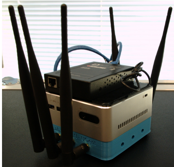
Figure 3: 3D printed antenna mount (blue colour)
