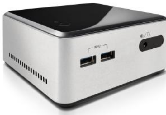
Figure 1: New portable testbed server (11 x 11 x 5 cm)
