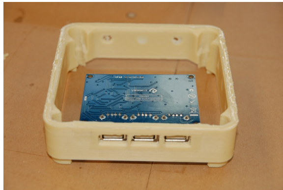
Figure 6: Antenna mount with Yepkit USB hub
