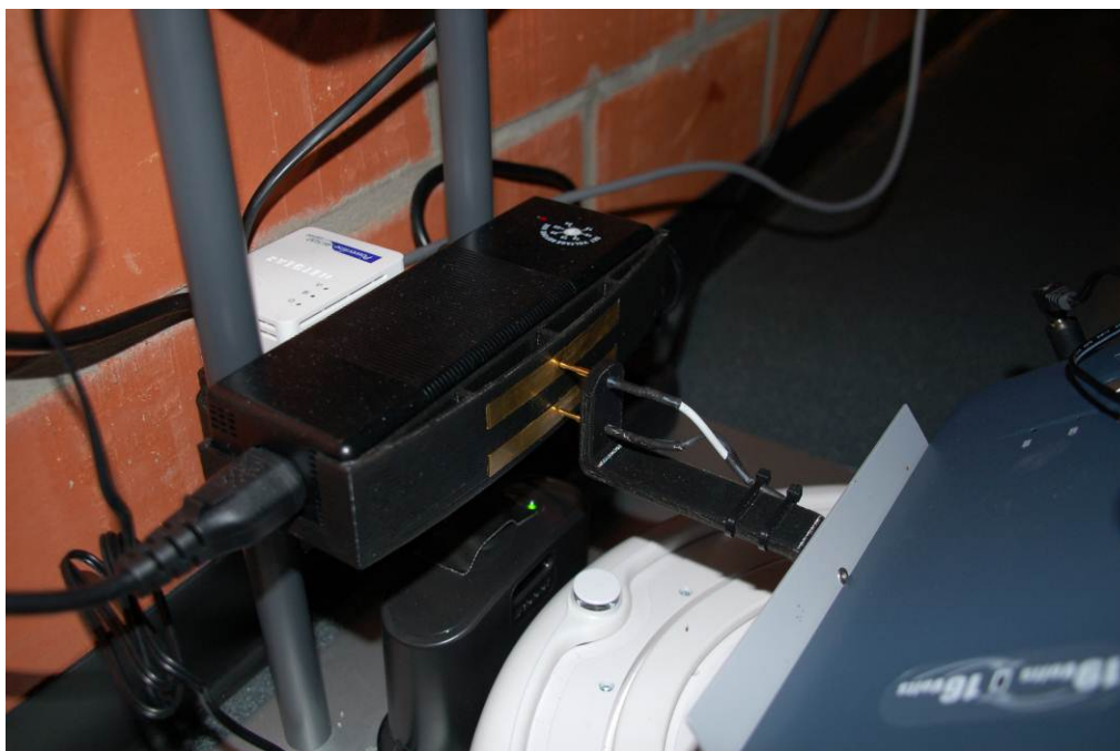
Figure 11: Pogo pins on a mobile node in IMINDS w-iLab.t
