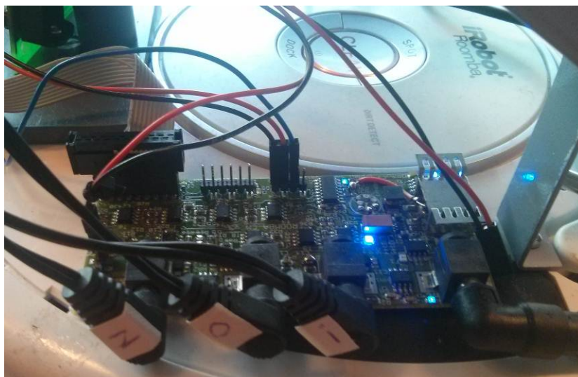
Figure 14: Power control (Chassis Manager) card on a robot in w-iLab.t
