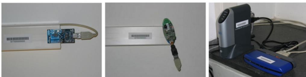
Figure 8 Tmote Sky (left), eyes IFXv2 (middle) and NLSU2 supernode / USB Hub (right).
