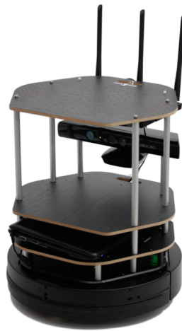
Figure 11 The Turtlebot Robotic Platform.
