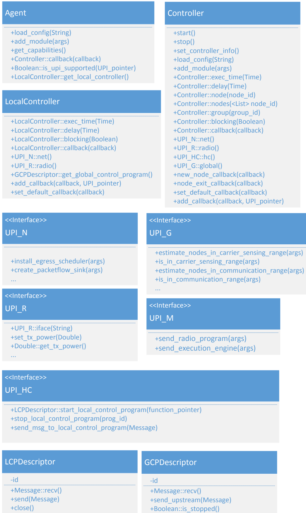
Figure 6. WiSHFUL control framework (UML class diagram).
