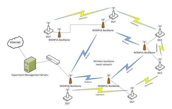
The **portable testbed** offers almost identical functionality to the experimenters as if they would run their experiments on one of the fixed testbeds:
